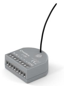
Receiver designed for radio control of a drive-in or garage door. The extended protocol of **COSMO | 2WAY** bi-directional communication and the use of additional sensors (contractors) facilitates sending the feedback about the position.
