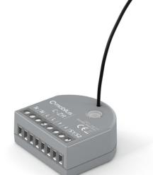
A concealed receiver for radio control of ordinary blinds motors. **MOBILUS C-ZR** enables the control of blinds position and inclination angle of slats. The extended protocol of COSMO | 2WAY bi-directional communication facilitates sending the feedback about the position or overload.
